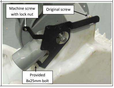
**5.** Attach SureDrive gear motor to bracket using socket head cap screws. A 5mm hex key is required for this procedure.
